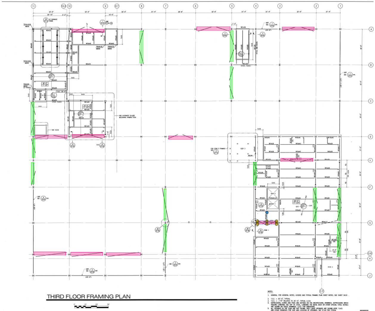
Third Floor Framing Plan Sheet S2.04 Showing BRB Frames, including Many that do not Engage Third Floor Framing
