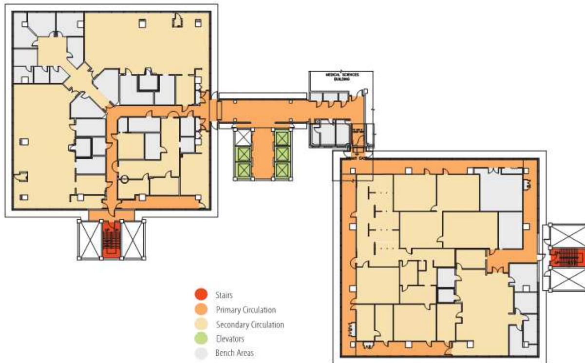
Figure 105: Circulation diagram for a typical laboratory floor. The building utilities and infrastructure scope U0 protects the primary circulation path to the mechanical tower stairs.
