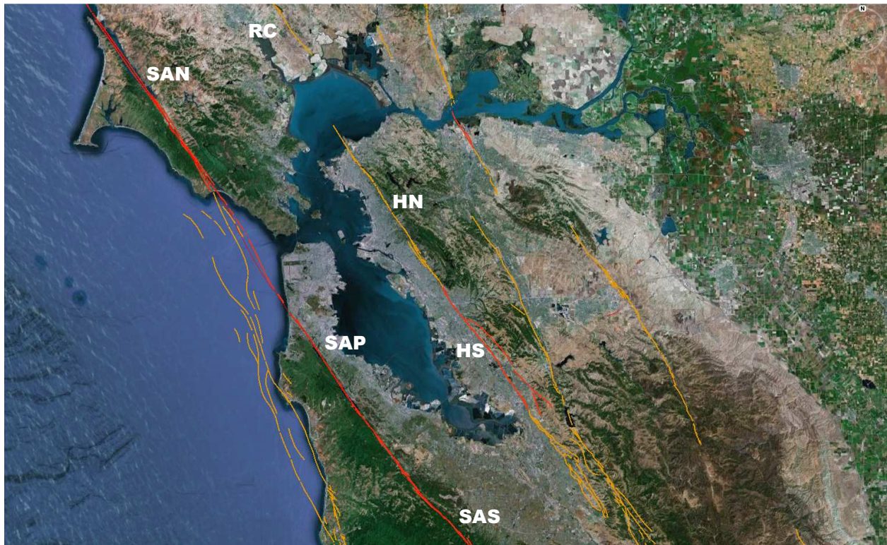
Figure 123: Fault segments considered in the Hayward and San Andreas ground motion scenarios. Key for Hayward-Rodgers Creek scenario: HS = Hayward South, HN = Hayward North, RC = Rodgers Creek. Key for San Andreas scenario: SAS = Santa Cruz Mountains segment, SAP = Peninsula segment, SAN = North Coast segment, SAO = Offshore segment (not shown). © 2012 Google. © 2012 TerraMetrics
